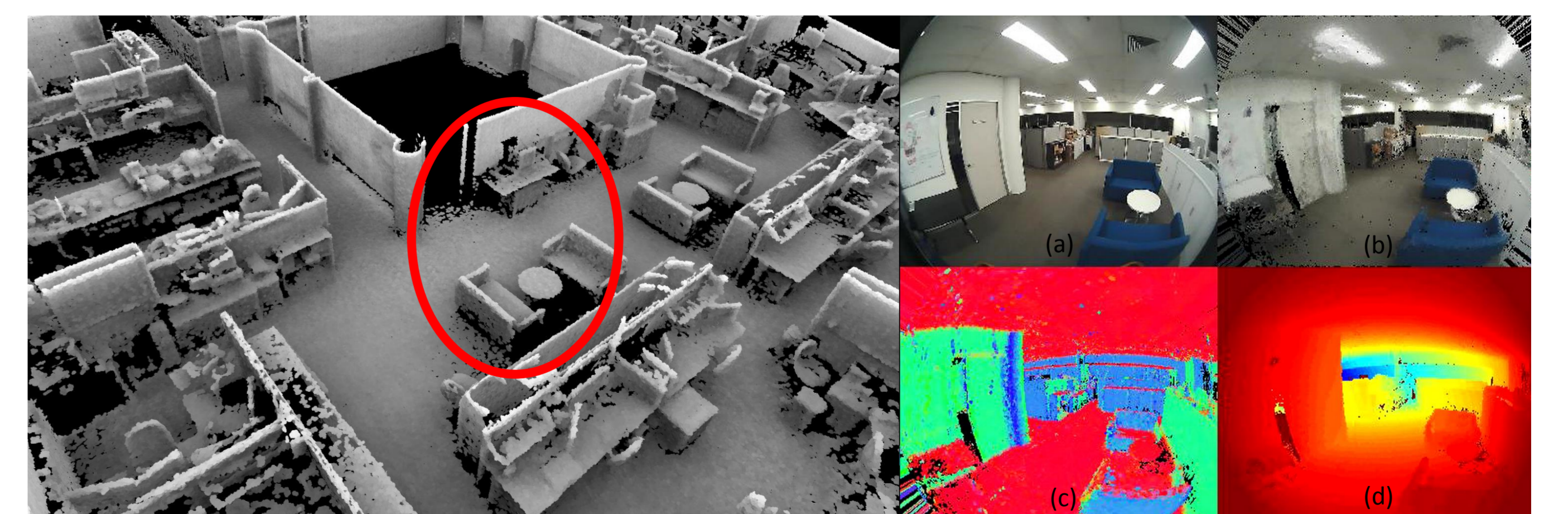
Figure 11: [Left] Reconstructed 3D surfel map of a 20x20 meter office. The details of the reconstructed map around the circled area is shown on the right side. [Right] (a) Raw camera image of the office around the red circle. (b) Synthesized image from the surfel map. (c) Surfel map colored with normal direction. (d) Rendered depth image from the surfel map.
