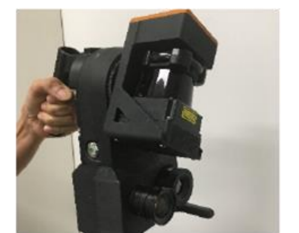
Figure 10: The experimental handheld 3D spinning LiDAR for mobile mapping.
